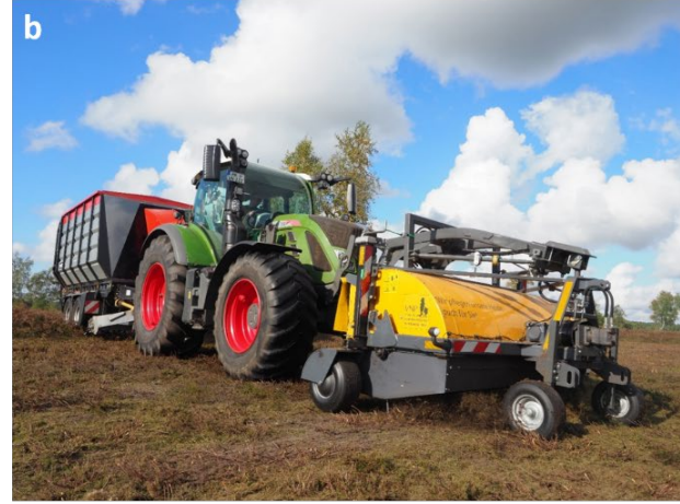
Left: Experimental site after scarification. Right: Using the newly developed scarification machine (© VNP Archiv, Dirk Mertens).
