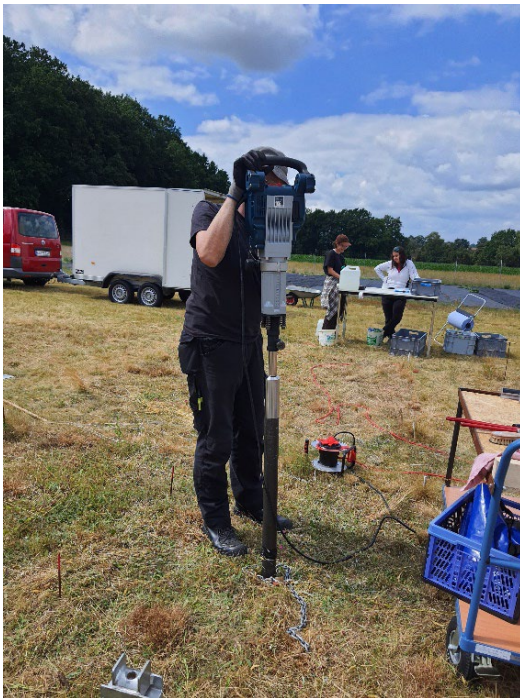
Pile-driving core probe with electric demolition hammer to take core probes.
