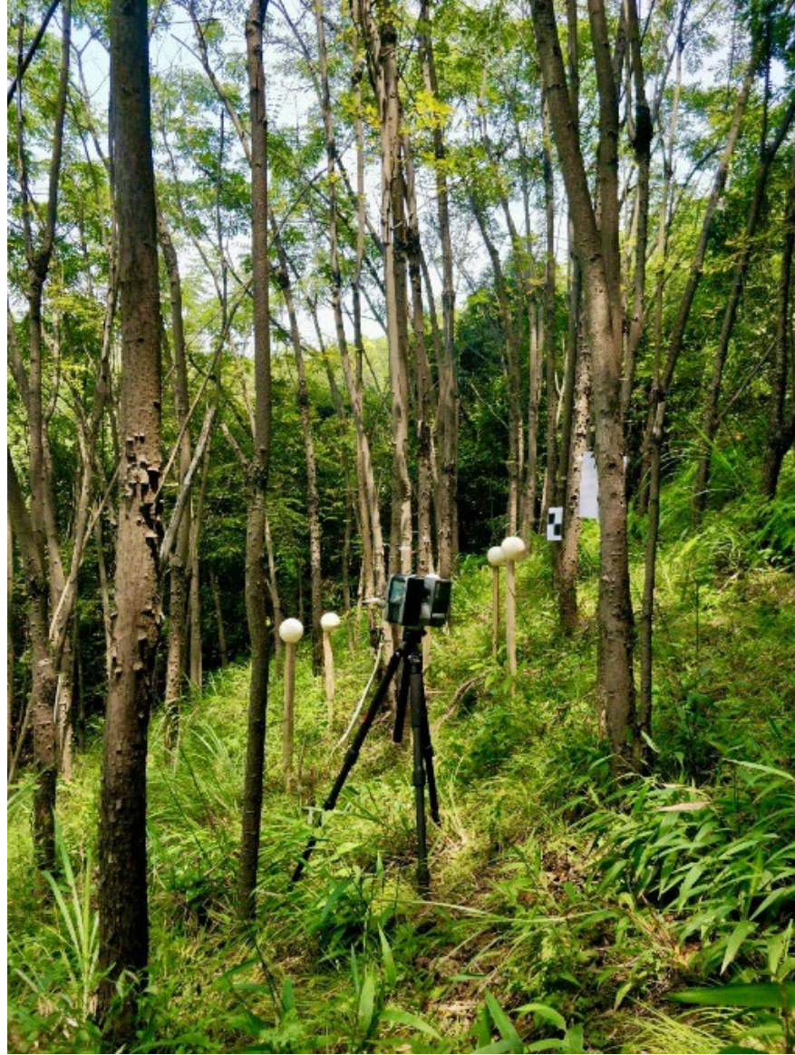
Terrestrial laser scanning of an experimental plot of the BEF-China experiment (©Tama Ray)
