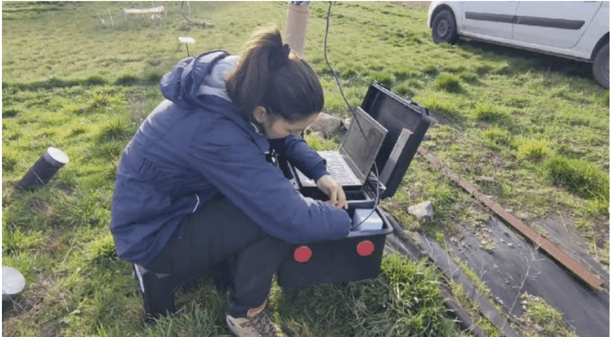
Minirhizotron images. Inés M. Alonso-Crespo taking MR images in POEM2021 experimental plots (© Inés M. Alonso-Crespo).
