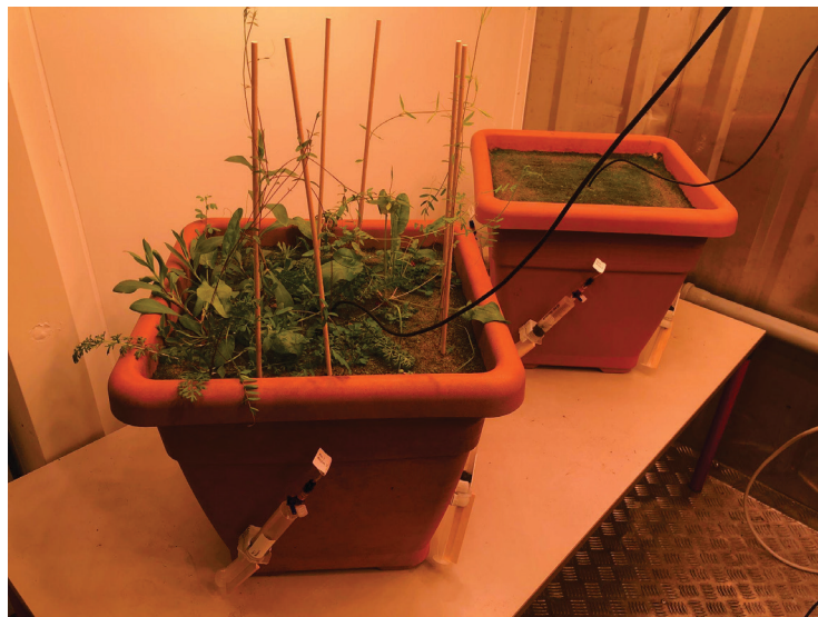
Experimental setup used to collect soil solution samples from dry grassland plant communities.
