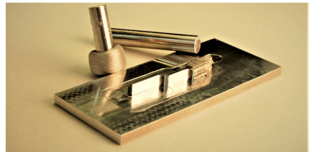
Demonstrator for the solid state layer deposition (SSLD) process showing multiple layers in as welded (right) and machined (middle and left) condition with used (background left) as well as unused (background right) friction surfacing studs. Source: HZG.
