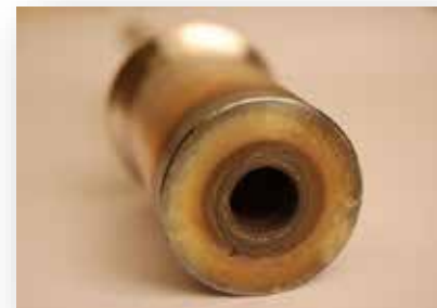
Single hole geometry steel demonstrator for the tube to tube sheet (TTS) hybrid friction diffusion bonding (HFDB) process.
