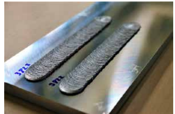
Aluminium substrate plate showing two parallel aluminium friction surfacing (FS) layers in as welded condition.
