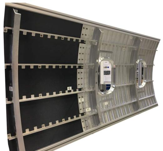
Hybrid metal-composite aircraft fuselage demonstrator joined entirely with friction-based processes. Build at HZG / Solid State Joining (WMP)
