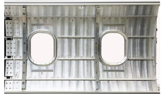
Aircraft demonstrator produced by using friction-based welding, including Refill FSSW
