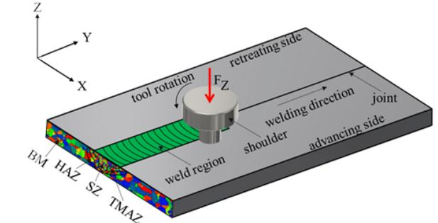
Schematic illustration of the FSW process, indicating the different zones of the microstructure appearing typical during the process (SZ: stirred zone; TMAZ: thermo-mechanically affected zone; HAZ: heat-affected zone; BM: bulk material)
